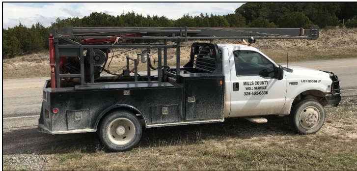
Water well workover rig
